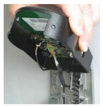
Plug the battery cable into the 2 pole connector terminal and the connection cable into the 6 pole connector terminal.
