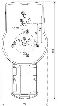
Drill the 3 fixation bores Ø3.2 x 14 mm and the cable leadthrough bore Ø10 mm. Remove burrs. Tap M4 threads into the 3 fixation bores.
