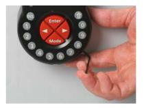
Check battery compartment for proper movability: carefully push the battery compartment into place, then slide it out again
