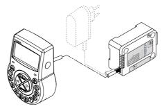
In its standard version the electronic safe lock Axessor IP is battery powered and consist of: the **input unit**, the **lock** and the **connection cable**. The lock includes 2 inputs and 2 outputs (assignment  $\rightarrow$  *External connections at the lock on page 24*). Optionally, an external power supply (6VDC/500mA) can be connected to one of the lock sockets "X1" or "X2".
