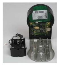
4. Fix the base plate with the enclosed special M4x12 flat-head screws to the door. The Input unit must be fixed to the door with at least two oppositely positioned screws. The third screw (Pos. 1) is recommended.
