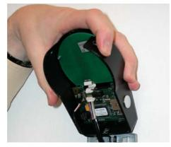
Slowly flip down the cover onto the base plate while carefully pulling the connection cable towards the lock chamber; leave some spare loop.
