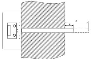
Fig. 4: Cutting to size of the actuating spindle
