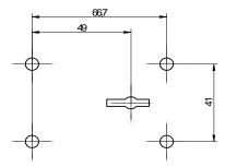
Fig. 3: Mounting hole pattern
