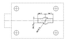
Fig. 2: Maximum cross sectional area of keyhole
