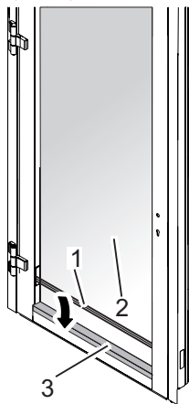
Fig. 37: Mounting the glass clamping profile
