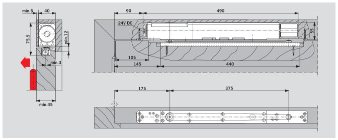
ITS 96 FL door closer with DORMA G 96 N20 slide channel in a timber door transom fixing. Example: Anticlockwise-closing (ISO 6) door; mirror image applies to clockwise-closing (ISO 5) doors.
