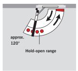
The RF hold-open unit enables doors to be securely held without any fall-back at precisely the required position up to an opening angle of approx. 120°. The pull-off force can be adjusted to any door situation. The RF mechanism is non-handed and has been specifically designed for retrofitting to the G 96 N20 slide channel.
