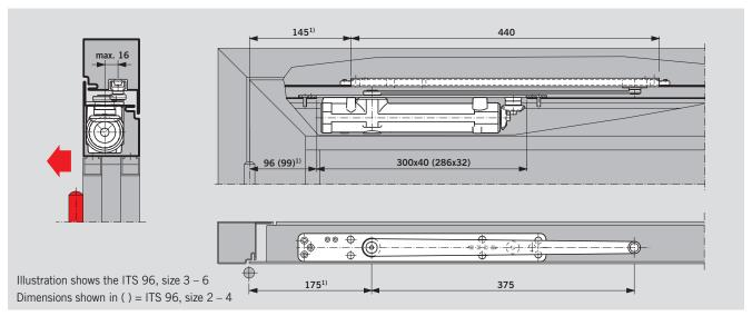
ITS 96 door closer with DORMA G 96 N20 slide channel in an **aluminium framed door.** Example: Anticlockwise-closing (ISO 6) door; mirror image applies to clockwise-closing (ISO 5) doors. <sup>1)</sup> Add 25 mm for aluminium profile frames with corner-angle reinforcement.
