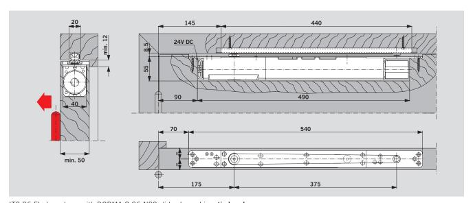
ITS 96 FL door closer with DORMA G 96 N20 slide channel in a **timber door.**Example: Anticlockwice closing (ISO 6) door mirror image applies to clockwice closing
