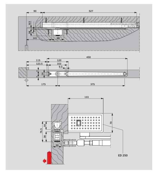
The pivot bearing used in conjunction with the G 96 N20 slide channel also acts as a cushioned limit stay.
