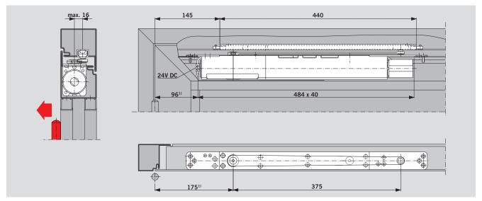
ITS 96 FL door closer with DORMA G 96 N20 slide channel in an **aluminium framed door**. Example: Anticlockwise-closing (ISO 6) door; mirror image applies to clockwise-closing (ISO 5) doors. <sup>1)</sup> Add 25 mm for aluminium profile frames with corner-angle reinforcement.
