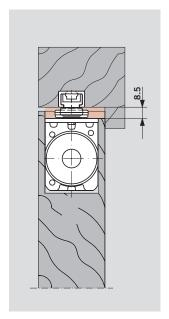
Timber door with steel frame, flush closing, clearance 12.5 mm, with ITS 96/ITS 96 FL EN 3–6, 4 mm extended spindle and slide channel G 96 N20 K8.
