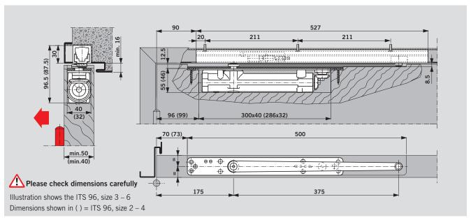
ITS 96 door closer with DORMA G 96 EMF slide channel assembly in a timber door.
