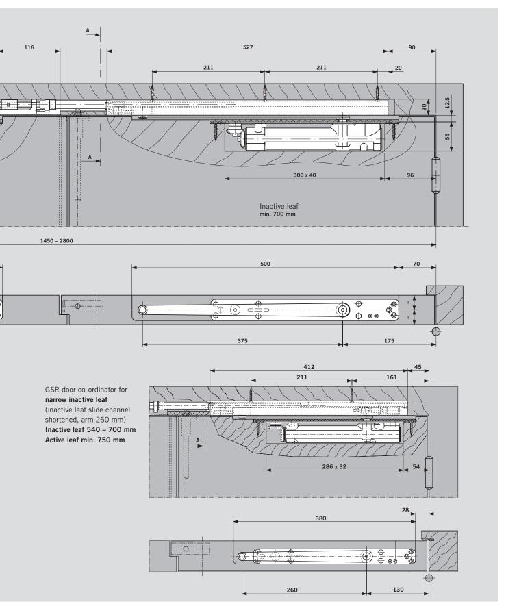
• When installed in fire and smoke check doors, ensure that the DORMA MK 397 carry bar is also fitted.
