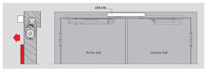
$\,$  RMZ frame-mounted smoke detector on the pull side connected to an ITS 96 FL GSR.
