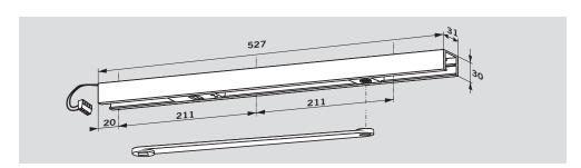
The slide channel assembly enables the door to be held open securely at a pre-selected position without fall-back.
