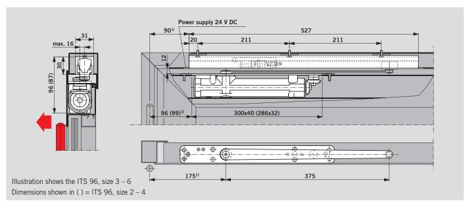
ITS 96 door closer with DORMA G 96 EMF slide channel assembly in an aluminium framed door.
