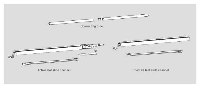
A G 96 GSR slide channel door co-ordinator encompasses an active leaf and an inactive leaf slide channel with electromechanical hold-open, a connecting tube, a cover for the co-ordinator mechanism on the active leaf slide channel, and two arms.
