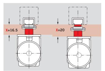
ITS 96 2-4 ITS 96 3-6 ITS 96 FL 3-6 with 8 mm extended spindle Timber door, flush-closing, clearance 8.5 mm, with ITS 96/ITS 96 FL EN 3–6 and slide channel G 96 N20 K8.
