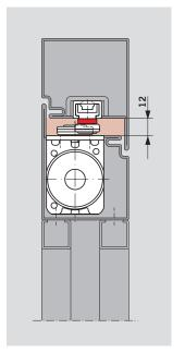
Aluminium tubular frame door, flush-closing, clearance 16 mm, with ITS 96/ITS 96 FL EN 3–6, 4 mm extended spindle and slide channel G 96 N20 K12.
