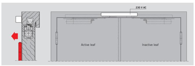
RMZ frame-mounted smoke detector on the pull side connected to an ITS 96 GSR-EMF.
