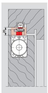
Hollow steel door with steel frame, over-rebated, clearance 12 mm, with ITS 96 EN 3-6, 4 mm extended spindle and slide channel G 96 EMF K8.
