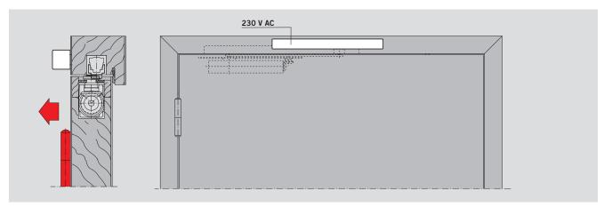
$\,$  RMZ frame-mounted smoke detector on the pull side connected to an ITS 96 EMF.
