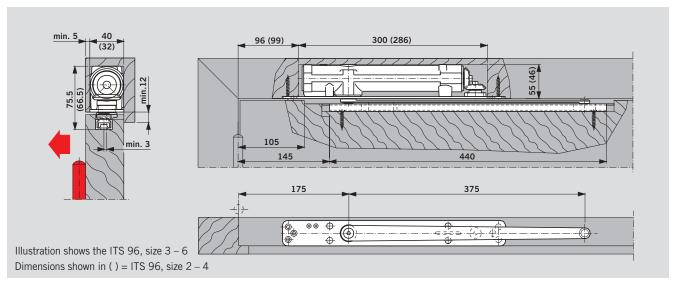
ITS 96 door closer with DORMA G 96 N20 slide channel in a timber door transom fixing. Example: Anticlockwise-closing (ISO 6) door; mirror image applies to clockwise-closing (ISO 5) doors.
