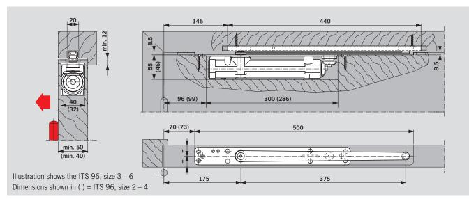
ITS 96 door closer with DORMA G 96 N20 slide channel in a timber door.
