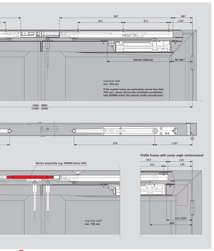
When installed in fire and smoke check doors, ensure that the DORMA MK 397 carry bar is also fitted.
