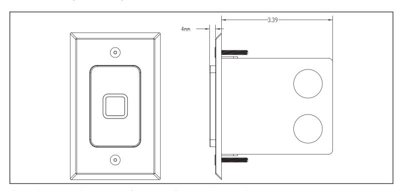
The reader must reside a minimum of 30cm away from any other RFID device.
