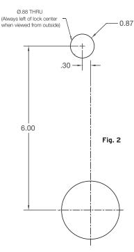
Note: The hole shown above is not located on the drill fixture. Use these measurements to locate the hole.
